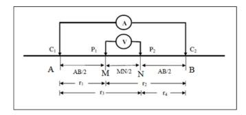
Figure 2. Electrode Arrangement of the Schlumberger Configuration (Modified Loke, 2004)
