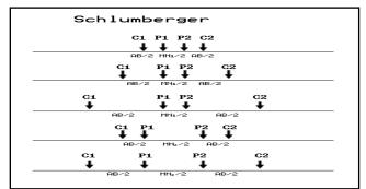
Figure 3. Electrode Displacement of the Schlumberger Configuration (Modified Loke, 1999)
