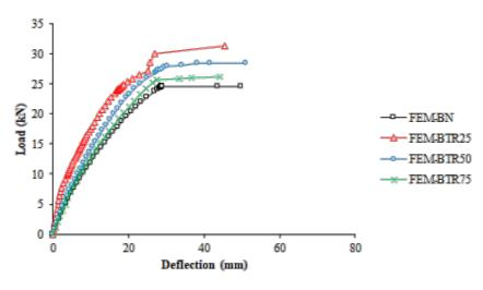
Figure 8. Load-deflection of the FEM results
