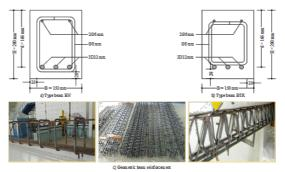
Figure 4. Detail of concrete beams
